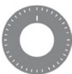
Incremental encoders generate an output signal each time the shaft rotates a certain amount. The number of signals per turn defines the resolution of the device.
