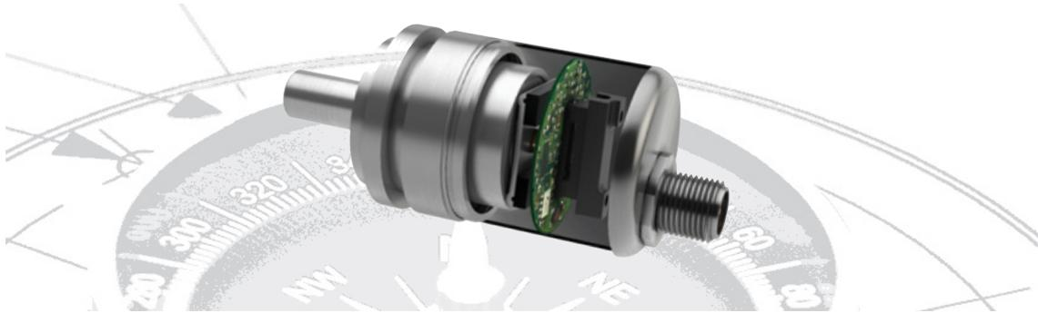
Magnetic rotary encoders determine angular position using magnetic field sensor technology. A permanent magnet **A** fixed to the encoder's shaft creates a magnetic field which is sampled by a sensor **B** that generates an accurate absolute position reading.
