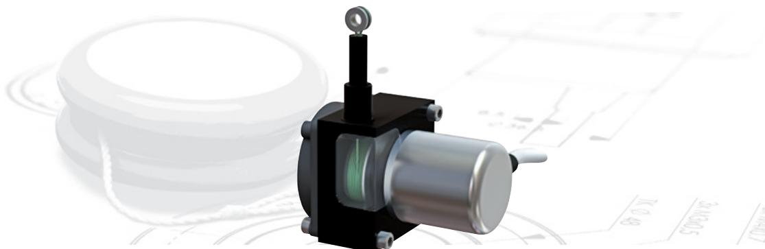
POSITAL's LINARIX draw wire sensors measure linear motion by displacing a retractable stainless steel wire **A** wound around a cable drum **B** that actuates the rotary encoder **C** coupled to it. The encoder then provides a proportional output. Measurements are highly accurate, reliable and the systems have very long lifetimes.
